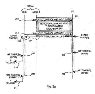
Figure 2a shows a communication situation in which an embodiment of the invention is applied: During time period 201, a radio link is established between the base station (left side) and a mobile station (right side). At time 204, the loss of the radio link is detected. Thereupon, two timers are started in the mobile station. The first of these is set to a relatively short elapsed time, which extends to time 206 and is typically
